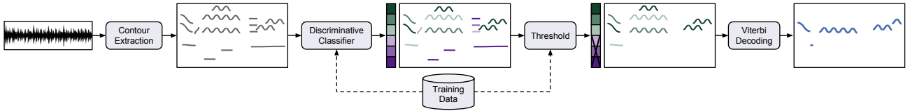
Figure 1. Block diagram of the proposed system (left to right): pitch contours are extracted from an audio signal, a classifier is used to score the contours and remove those below a threshold, the final f_0 sequence is obtained using Viterbi decoding.
