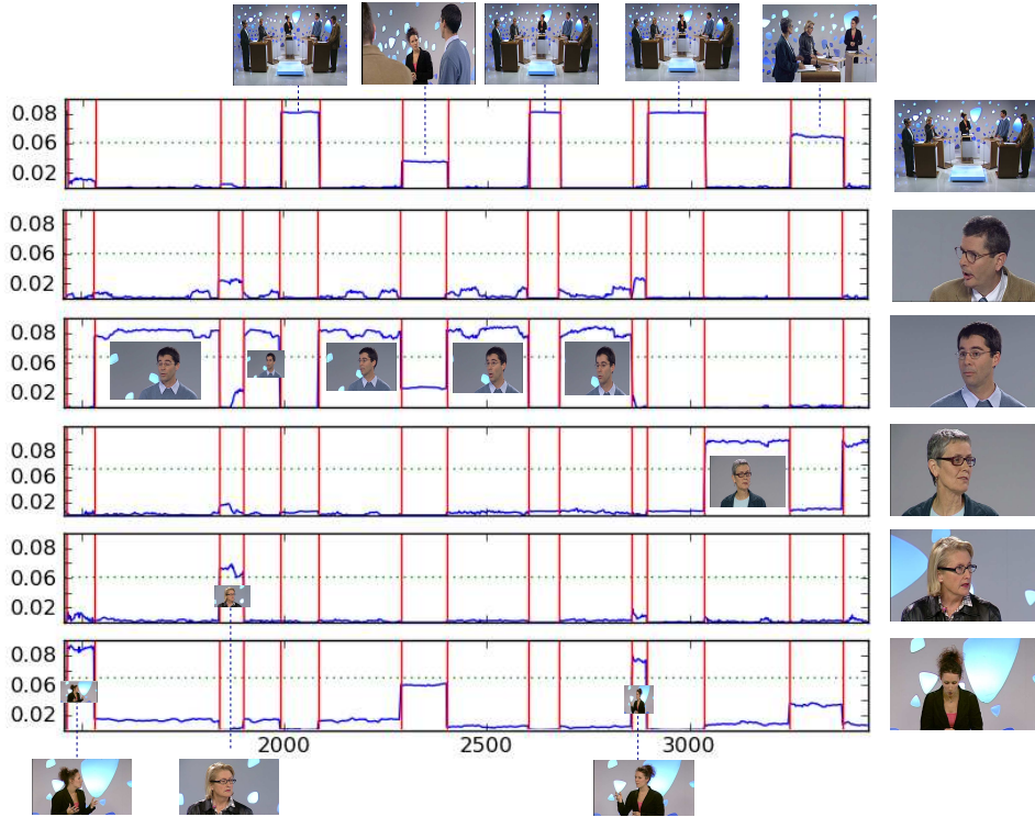
Figure 3: KL-NMF activations, i.e., H coefficients on a short excerpt of the development video with \beta = 0 . Each subplot represents the temporal sequence of activations for one w_k component, 1 \leq k \leq K = N_{sp} + 1 . For each component, the image on the right corresponds to the frame where the activation value is maximum, which is supposed to be a good representative of the content modeled by the corresponding w_k component. Red vertical lines are groundtruth shot boundaries and the other images inside the plot or around it are key frames of the time-corresponding shots. Green dotted horizontal lines are decision thresholds. It can be seen that NMF has succeeded in extracting the relevant components and related activations. Note that the 2nd component is not activated here as the corresponding person does not appear in any personal shot of this part of the video.
