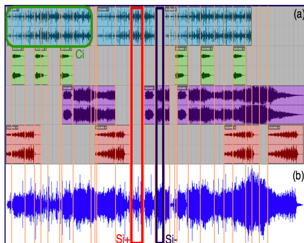
Fig. 2: Time-line representation of a polyphonic piece with C_i (target class), S_{i+} (initial positive segment) and S_{i-} (initial negative segment). Though the distinct sound layers are here displayed in parallel time lines (a), in real situations the user can actually only see the final mix made by the composer that appears as a single track (b). The initial user selection and subsequent validations are done by listening.
